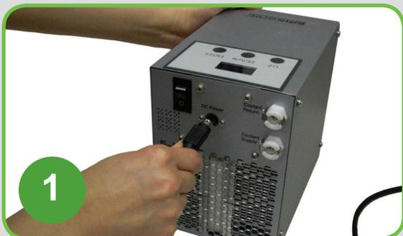
Connect the *Power Adapter's* cord to the back of the *Recirculating Chiller*.
