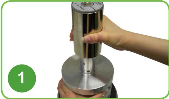
Lay *Sample Processing Horn* upside-down on a flat surface. Carefully attach converter by tightening clockwise with hands.
