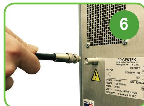
Connect and fasten the other end of the *Converter Cable* to the rear panel of the *Sonication Generator*. Make sure it is securely attached by turning the fastening mechanism clockwise at the end of the cable.
