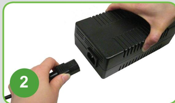
Connect the *Power Cord* to the *Power Adapter*. Plug *Power Cord* into a grounded power outlet.
