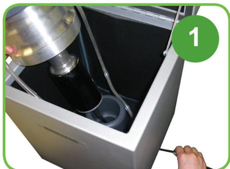
Open the lid of the *Soundproof Enclosure* and feed the *Flow Tubing* through the two holes at the bottom of the *Soundproof Enclosure*. Feed the other end of the *Converter Cable* through the main opening at the bottom until you can rest the *Converter* comfortably and firmly in the opening.
