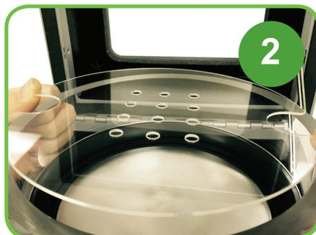
Place the *Tube Rack* into the *Sample Processing Horn* so that it rests on the gray inner rim inside the reservoir.
