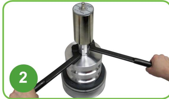
Firmly tighten with *Assembly Wrenches*. Rotate the top wrench clockwise and the bottom wrench counterclockwise.
