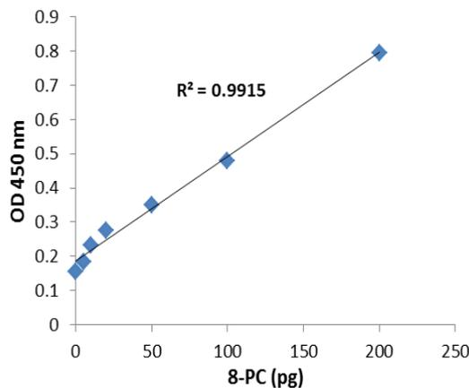
Fig 3. 8-NG standard control was added into the assay wells at different concentrations and then measured with the EpiQuik™ Nitrosative (8-Nitroguanine) DNA/RNA Damage Quantification Kit (Colorimetric)
