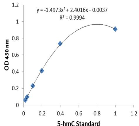
▲ Standard curve generated with use of the positive controls.
