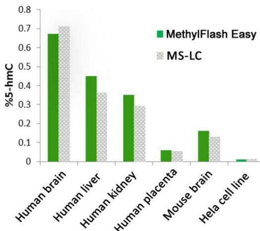
▲ Accurate quantification of 5-hmC content of various DNA samples from different species with the MethylFlash™ Global DNA Hydroxymethylation (5-hmC) ELISA Easy Kit. The results are closely correlated with those obtained by MS-LC.
