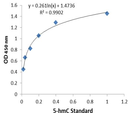
▲ Standard curve generated with use of the positive controls.
