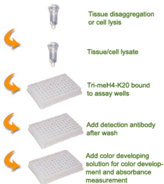
Schematic Procedure for Using the EpiQuik™ Global Tri-Methyl Histone H4-K20 Quantification Kit (Colorimetric)
