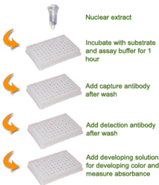
Schematic Procedure for Using the EpiQuik™ Histone Methyltransferase Activity/Inhibition Assay Kit (H3-K9)
