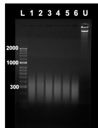
▲ Demonstration of consistent DNA shearing in different positions. 2 µg of HeLa DNA in 0.2 ml PCR tubes were inserted into the 0.2ml Tube Rack and processed with 20 sec on 30 sec off for 60 cycles at 20% amplitude. An average size of 250 bp is generated from DNA samples placed in different positions.
